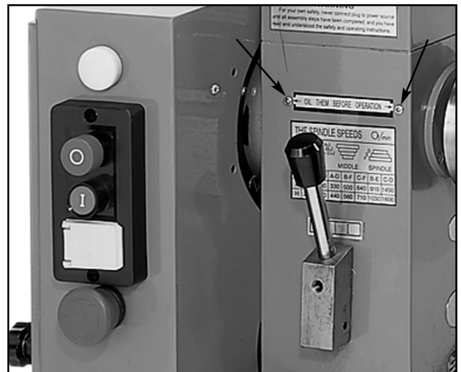
Figure 53. Gearbox lubrication points.
